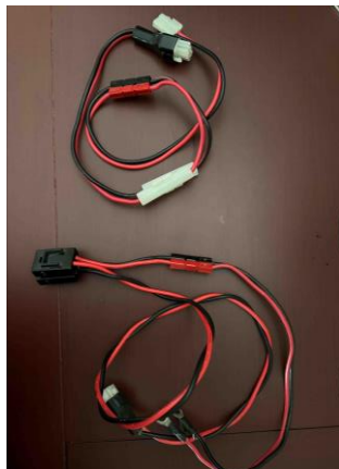
Top – DC power cable with Anderson Power Poles and older style “glass tube” fuse holders on both leads.
