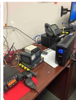
Exercise scenario's included loss of power requiring battery backup operations. Shown is a UPS on battery operation.
