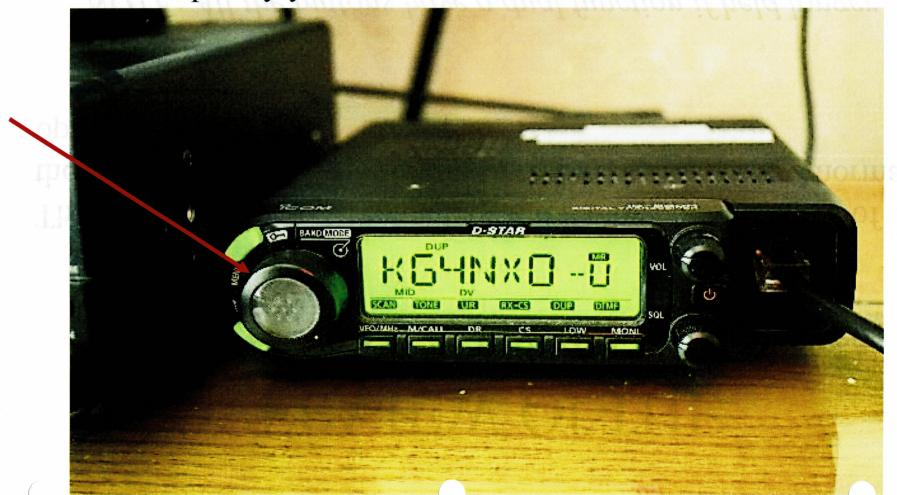
2. You turned the **TUNING DIAL** and the **REPEATOR NAME** is displayed but you cannot change to a different CHANNEL or FREQUENCY. You can only transmit and receive on this Channel/Frequency. **The RADIO is LOCKED**.
