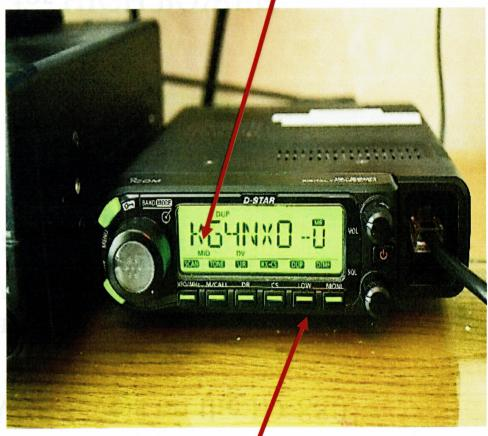
Press the LOW button less than 1 second to change the power level. 18
