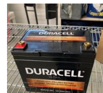
Replacement 35 Ah AGM radio batteries
