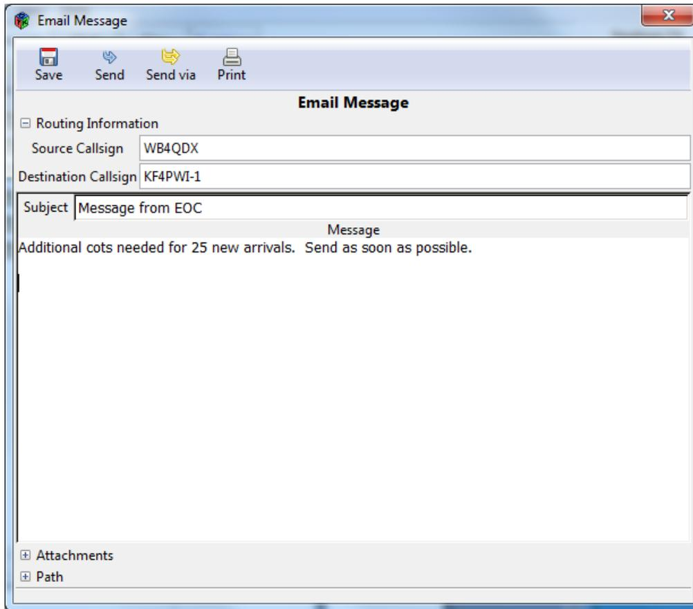
To send a form such as an ICS-213, select New and the desired form from the list. A standard ICS-213 form is included with D-RATS. Fill in the information and select Send. Only the contents of the form will be transmitted for efficiency and the form will be populated on the receiving end.
