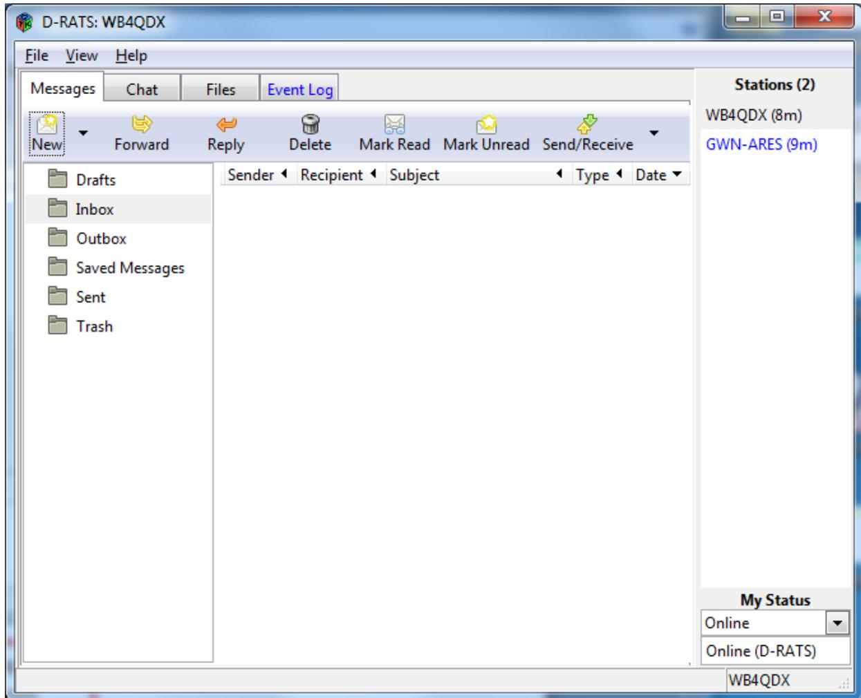
To send a regular message to another station, click New and either Memo or Email. Type in the Destination callsign . Remember, this can either be the actual callsign or a tactical callsign. To ensure the correct destination, ping all stations as in Chat and use the station name exactly as it appears. If the desired station is not online, you must still use the exact destination callsign, but the message will not leave your Outbox until the stations is online.
