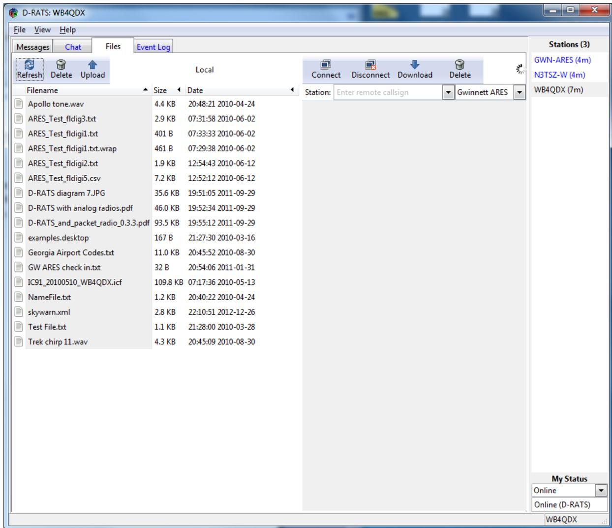
To download a file from a distant station, again make sure you are connected to that station. Click on the file on the right side of the screen highlighting the file and click Download. Again, the file transfer progress will be shown at the bottom of the screen. Be sure to Disconnect from the distant station when you are finished transferring files.
